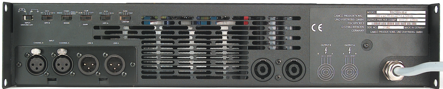
Backpanel of the power amp with switches for operating mode, gain and HP-filter for subwoofer/fullrange-cabinets.
